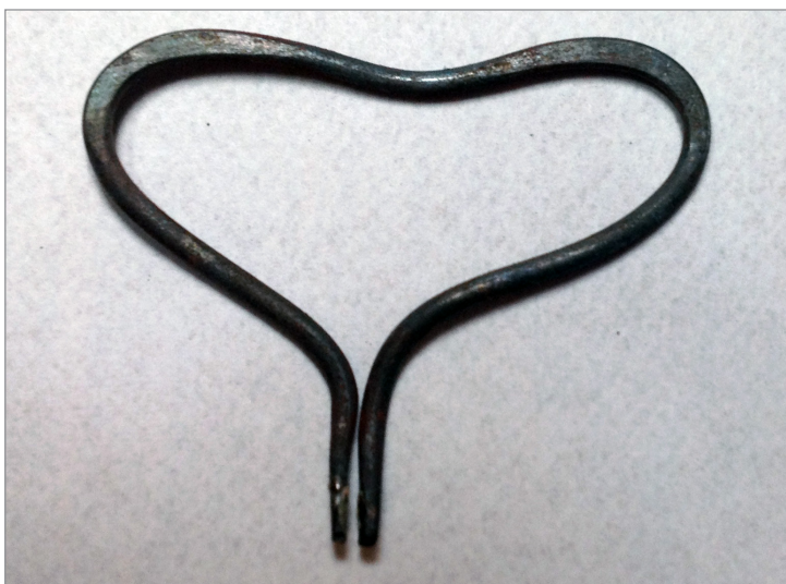
A tool, bent and forged out of iron, makes an ideal parts holder during soldering.
