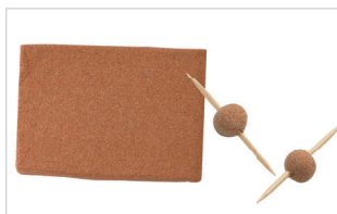
Use cork clay as a core when creating hollow PMC® objects.
