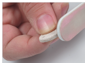
Manicure sanding boards are ideal for sanding and shaping.
