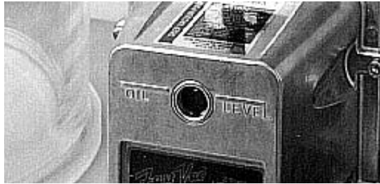
Fill pump to "full" mark on oil sight gauge.
