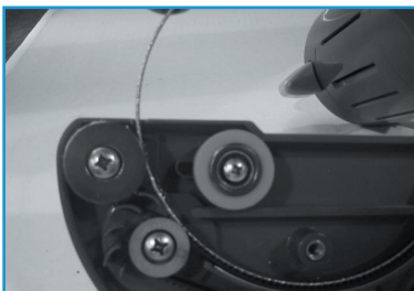
Loosen Groove Grommet #7 and slide it back. When replacing the blade, slide it forward until it makes contact with Groove Grommet #6.
