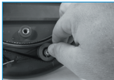
Lift up on tension arm #10 and slide drive belt off of blue pulley #4.
