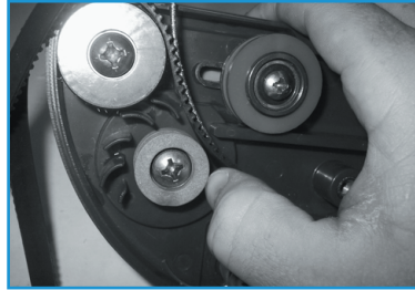
Slip drive belt and blade past blue pulley #5, then wrap the drive belt around it. From this point just follow the previous steps in reverse order.
