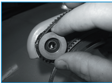
Wrap drive belt #9 around blue pulley #1 and slip them into position. Insert screw and tighten.
