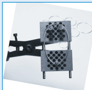
Squeeze the pliers to stretch the wire ring into a new shape.
