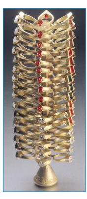
Setting stones into a wax model and casting metal directly around them can attain significant labor cost savings. This procedure requires several carefully monitored steps to avoid damage to the stones, including good form-filling at modified casting temperatures, minimal thermal shock, and controlled metal flow to achieve good results. The caster must understand the scientific principles involved in this procedure; otherwise it should not be attempted.
