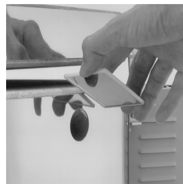
Vent the kiln until moisture no longer fogs a mirror.
