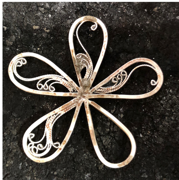
The solder applied to the filigree in the top petal
