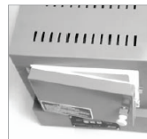
Open the door 1/2" to vent the kiln if your kiln does not have vent holes.
