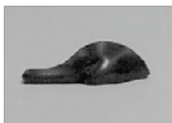
An over-fired cone with "puddled" appearance.
