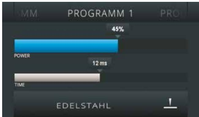
Pressing and holding the metal selection in the start menu or the welding curve in the expert menu results in the current parameters set being accepted in the program memory menu. 20 storage spaces are available here for individual storage. In the first step, the program space is selected by swiping to the left or right. The set data is then accepted by pressing the "continue" button. Saved data cannot be deleted. It can only be overwritten. A program name is assigned
