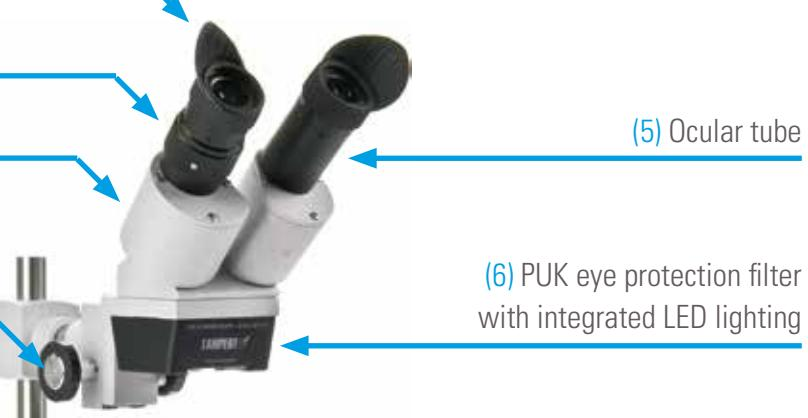
Look through the two oculars (1) and move the ocular tubes (5) inwards or outwards by moving the prism housing (3) in or out. The interocular distance is correct if the range of vision as viewed through the two oculars is complete and is united as a single complete image. The interocular distance should be individually set for each user. A spacer sleeve ensures the correct distance for focussing.
