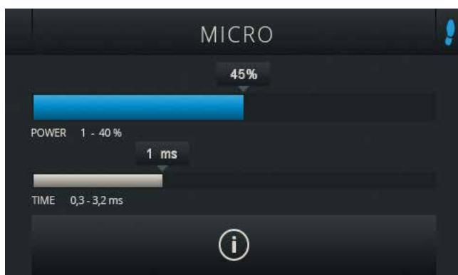
The micro menu can be activated in the settings user level. After activation, the micro menu appears as a separate user level, which can be accessed by pressing and holding the multifunctional controller. In micro menu the welding parameters can be adjusted much finer allowing the welding of wires and sheets with material thickness down to less than 0.2 mm with even greater control.
