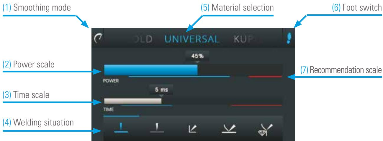
The smoothing mode (1) and welding situation (4) functions can be selected directly via the touch display by tapping with the finger. The power scale (2), time scale (3) and menu field (5) can be changed with the swipe function on the touch display. The recommendation scale (7) shows the recommended setting range. In the red range, the settings are no longer expedient and there is a possible risk of damaging the workpiece. The foot switch (6) can be activated by pressing it for 2 seconds.
