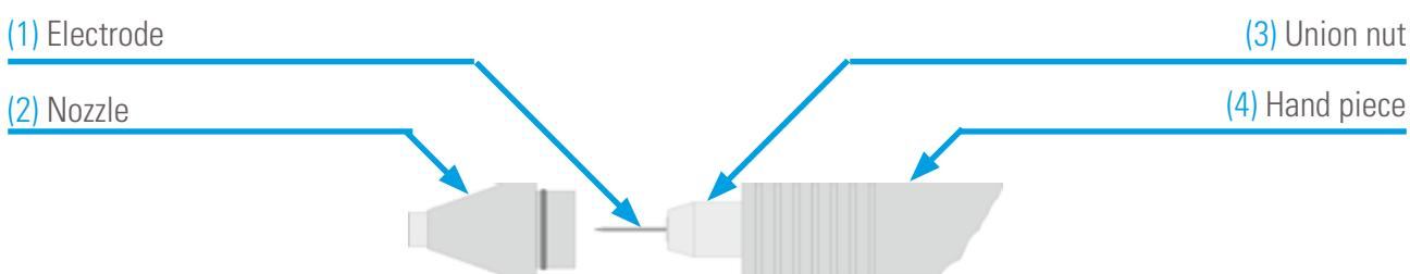
Lightly rotate the nozzle (2) and in doing so, pull it off of the hand piece (4). The nozzle is in place but not screwed on. Undo the union nut (3), remove the electrode (1) and insert the freshly abraded electrode with the freshly sharpened side facing outwards, tighten the union nut once more until hand-tight.
