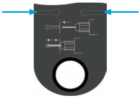
The correct electrode length can be easily set with the help of the measuring aid milled into the hand piece arm. Suitable for right and left-handed users.
