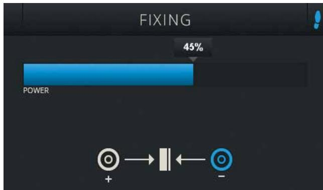
The fixation welding menu can be activated from the settings user level. After activation, the fixation welding mode appears as a separate user level, which is accessed by pressing and holding the multifunctional controller. This mode is used for workpiece fixation. The fixation welding set is required for fixation welding (optional accessories). Connect both of the workpieces which are to be fixed to an area of bare metal, using the blue and the black connection terminal respectively.
