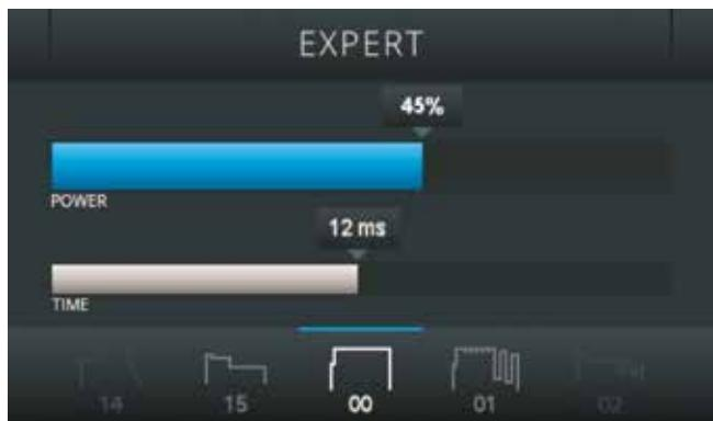
The expert menu can be activated in the settings user level. After activation, the expert menu appears as a separate user level, which can be accessed by pressing and holding the multifunctional controller. The various welding characteristic curves are stored in the expert menu, which have been developed and defined in the start menu for the preconfigured metals and welding geometries. However, here they are shown without content-related assignment. This mode is designed
