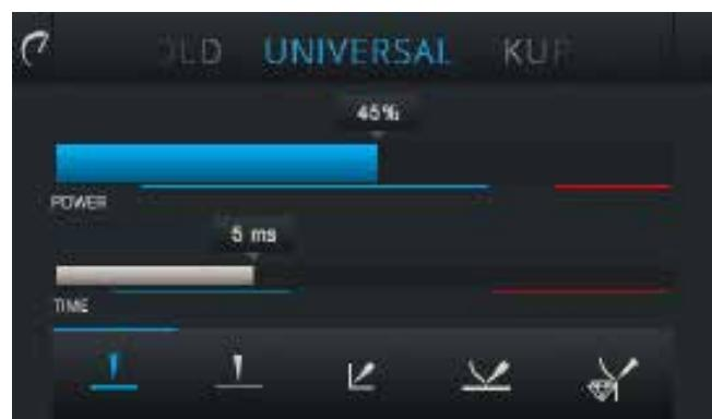
In the start menu user level, it is possible to start welding immediately. At the top edge of the display it is possible to select the welding material, and at the lower edge you can select the geometries or welding situations.
