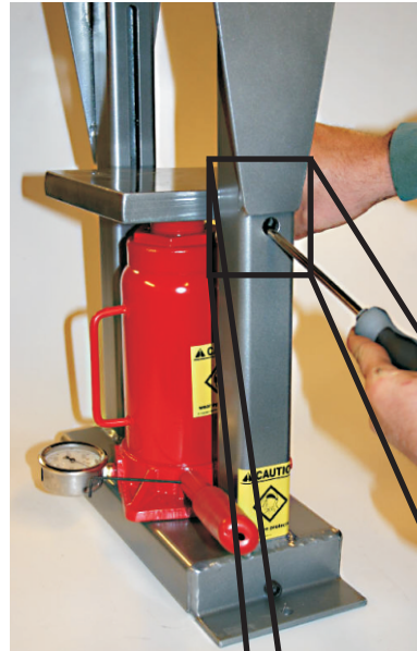
Figure 2 Lift the lower platen by using a screwdriver to pry the platen bolt upwards
