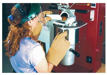
The J-2R gives you accurate temperature control and oxygen-free casting like our larger casting machines, but heats metal using electrical resistance. It's the perfect machine for small jewelry manufacturing operations.
