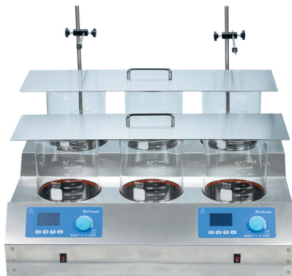
3-liter plating unit with lids in place over beakers
