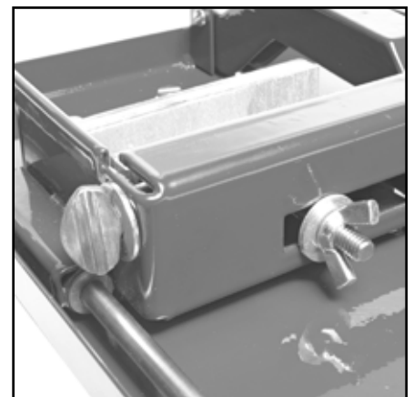
Fig 13 - Cross feed lock (right) and cross feed thumb screw (left)
