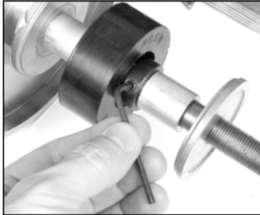
Fig 49 - Loosen the set screw that secures the right-side bearing collar
