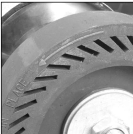
Fig 59 - Arrow on drum indicates direction of rotation
