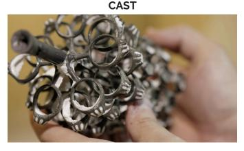
Jewelry pieces will need to be clipped and ground. Then, a cycle of pin finishing to remove casting scale and any residual investment. Cast pieces usually require medium and fine cut-down steps before a final finish. FABRICATED
