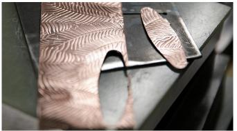
Most fabricated pieces may only require the burnishing cycle to smooth out the slight imperfections and rough edges left after sawing or punching.
