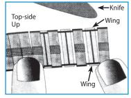
5. When the band is ready to be reassembled, place both sides together in front of you, top-side up. With long-nose pliers or tweezers, reinsert the U-shaped pins in the top and underside of the connecting band links. Bend the side wing back down on the top link and underside link.
