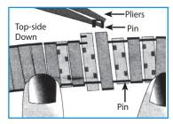
Remove the necessary number of links by repeating steps 1 through 3, beginning with the link next to the last link to be removed.
