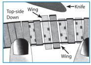
3. With long-nose pliers or tweezers, carefully pull out connecting U-shaped pins between adjacent links on the top side and the underside.
