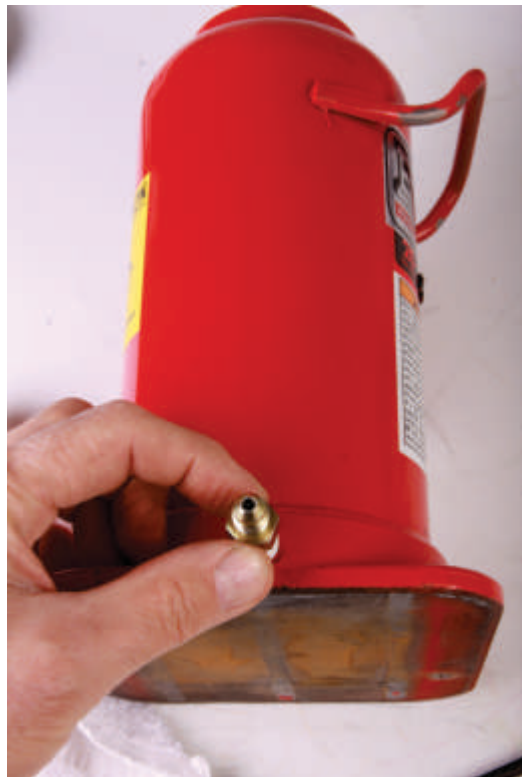
Hand thread the brass colored nipple into the port, hand thread only at least two turns.
