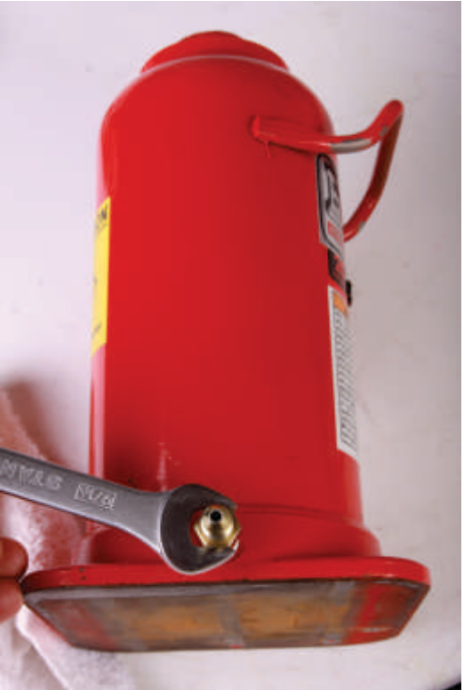
Only after hand threading should you tighten the nipple with a 9/16" wrench.
