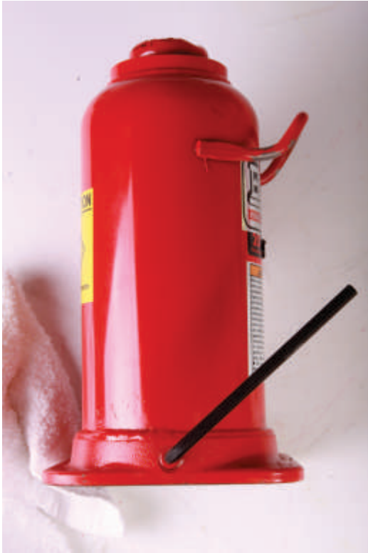
Lay the ram on it's side, have a rag or two handy to wipe up leaks.
