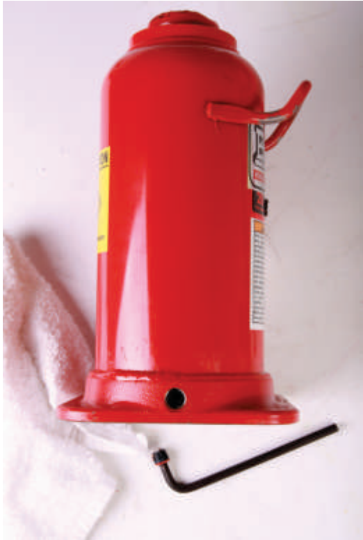
Use the supplied hex ket to undo the port plug at the base of the ram.
